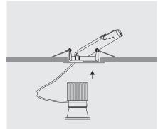
3. Gently insert module holder from the bottom of the fixture frame.
