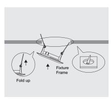
1. Cutout and fold up the spring clips and gently insert one side of the fixture into the cut out hole.
